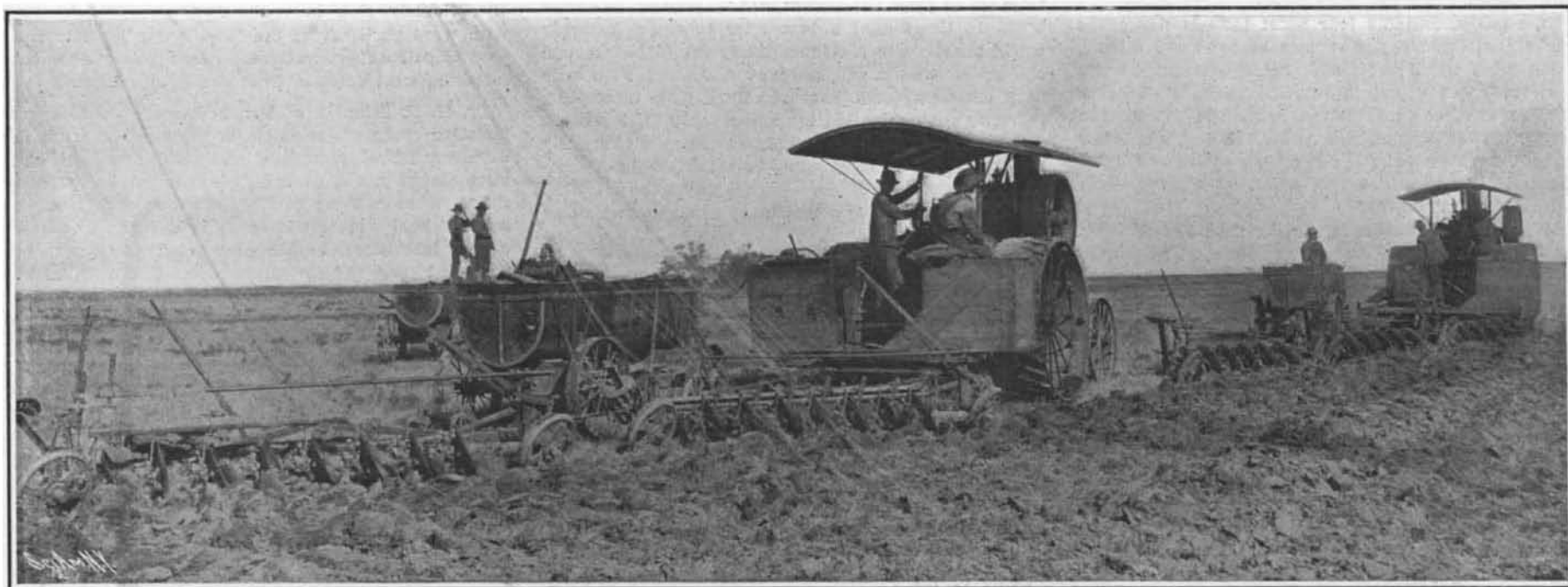
Breaking the Ground for Dry Farming. The Work is Done on a Large Scale, and Machine Power is Necessary. One Plowing Outfit Can Prepare 3,000 Acres of Sod in One Season.
