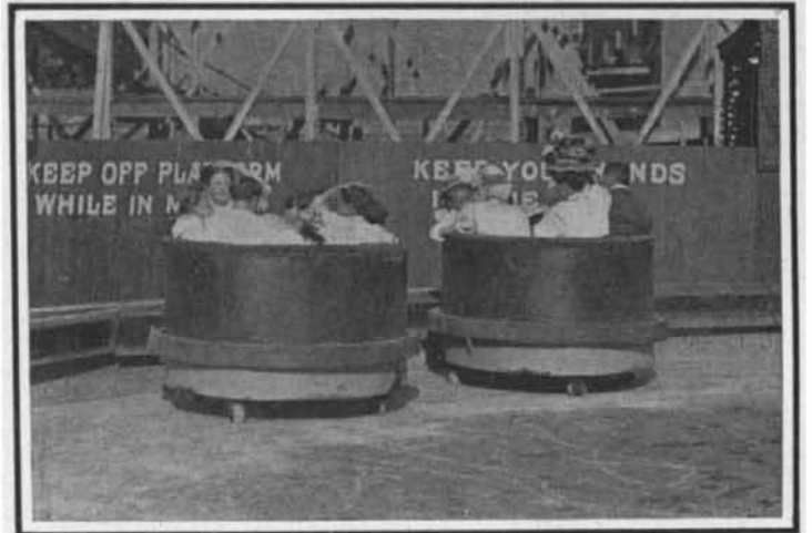
The "Scrambler." A Circular Rotating Floor Causes the Cars to Spin and Carom.
