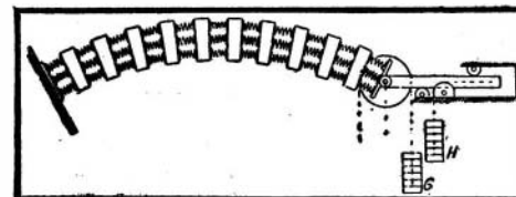
Fig. 7.—Diagram of arch with sliding abutment.
