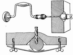
A METHOD OF DRILLING HOLES IN MARBLES.
