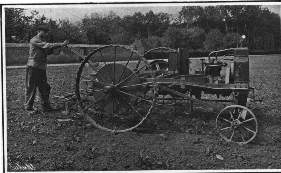
Fig. 3.—The automobile hoe with bonnet removed to show mechanism.
