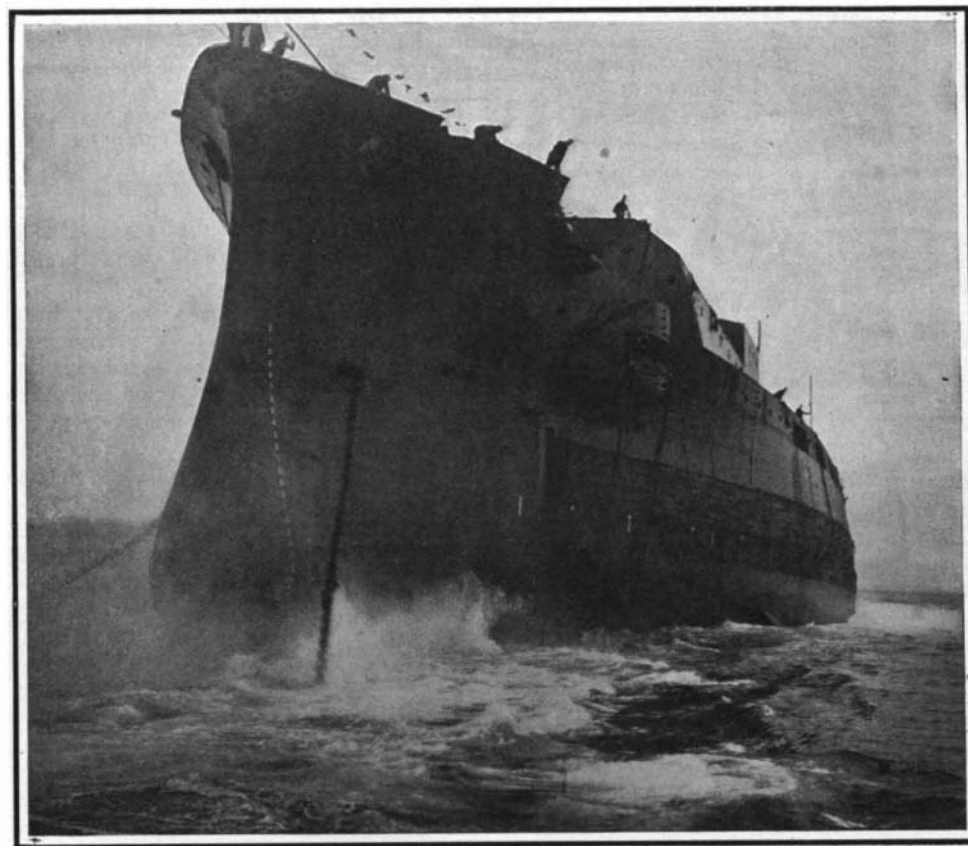
Displacement: 20,000 tons. Speed, 21 knots. Guns, ten 12-inch, fourteen 5-inch. Note the lofty fore-castle deck and flaring bow.
