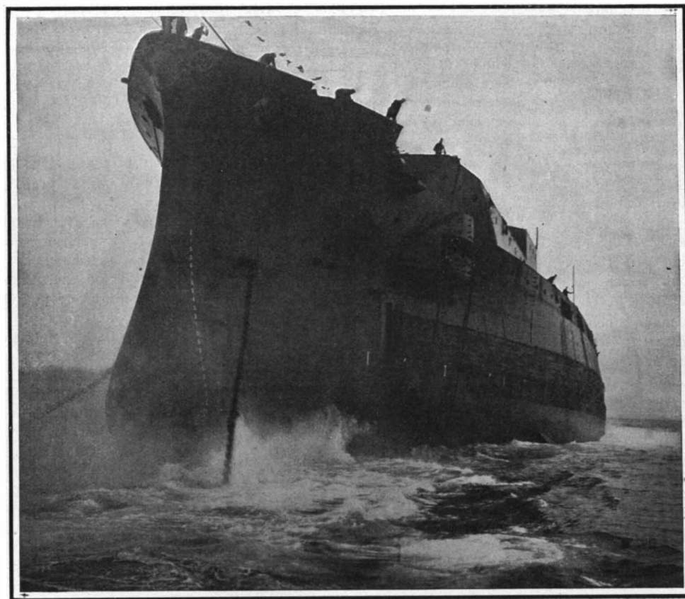
Displacement: 20,000 tons. Speed, 21 knots. Guns, ten 12-inch, fourteen 5-inch. Note the lofty forecandle deck and flaring bow.
