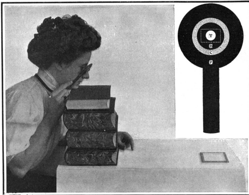
The invisible printing is read easily through what appears to be common green glass.
