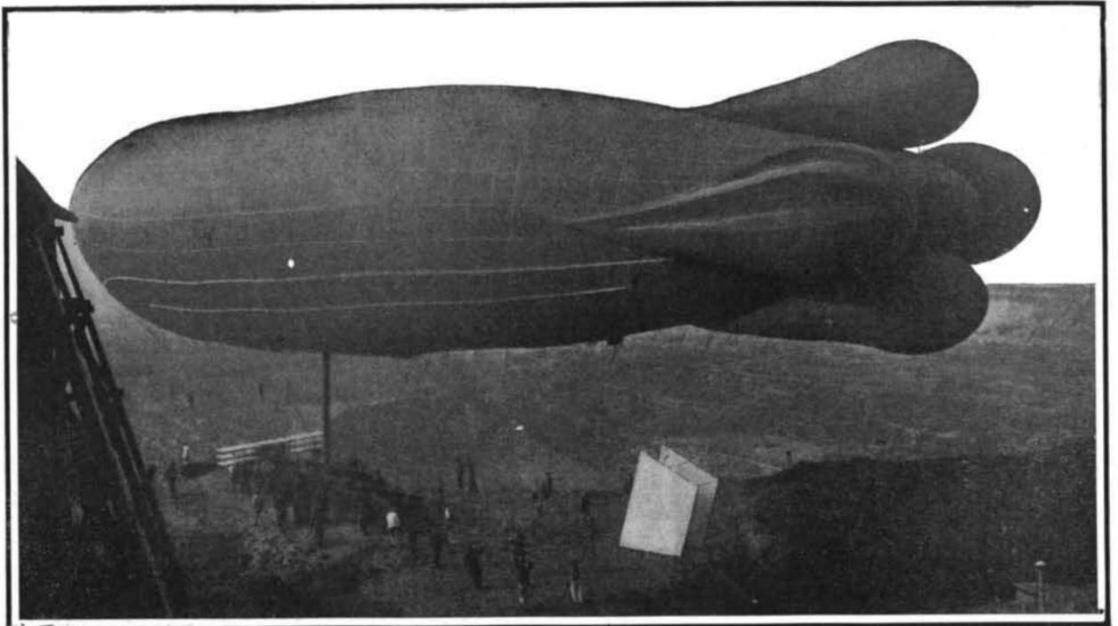
**The new Clement airship, showing the peculiar tail, the propeller, and the horizontal and vertical rudders.**
