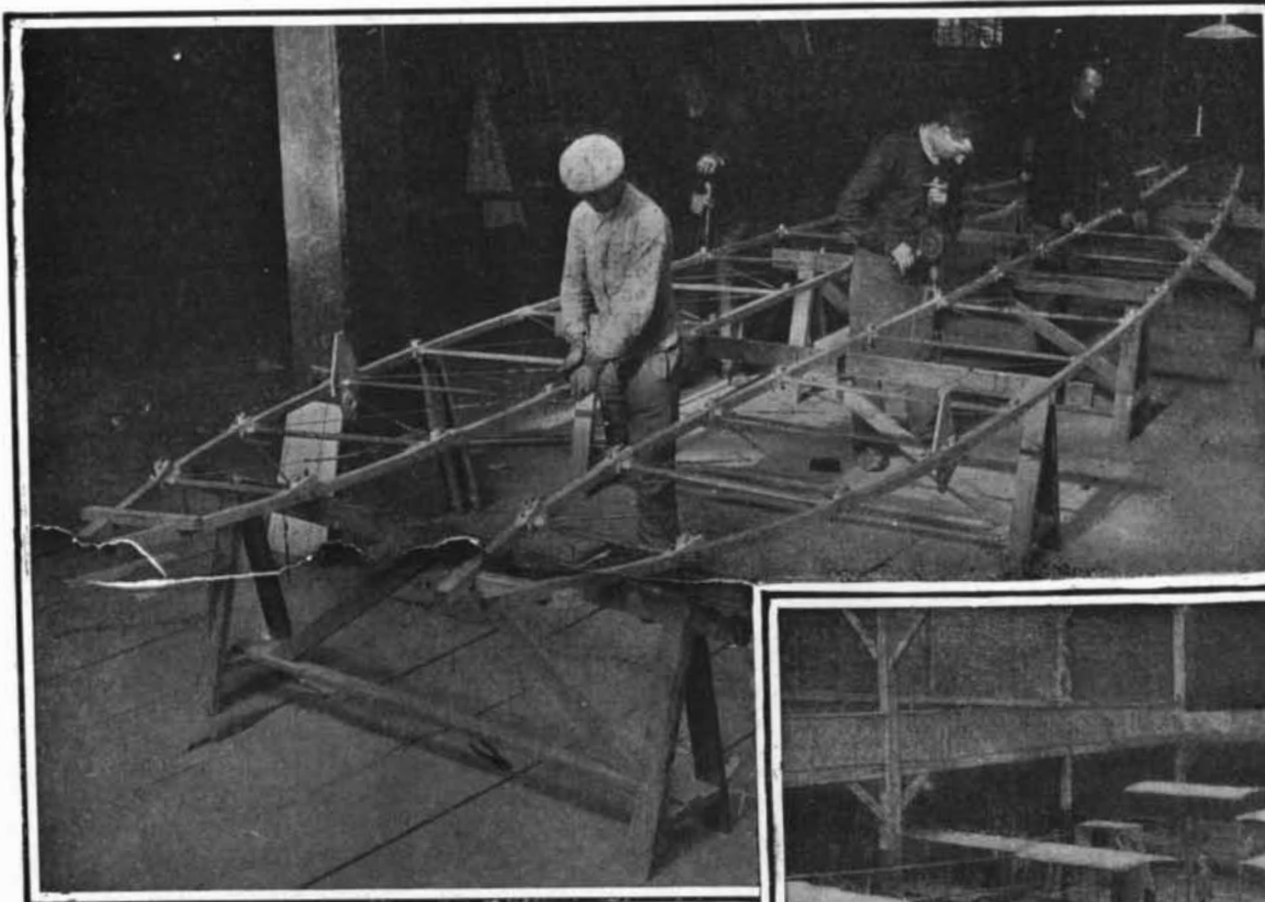
Side members of the main body frame of an aeroplane.
