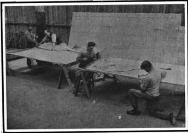
Covering the frame of a plane with cloth.
