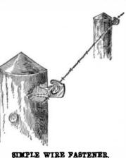
to prevent it from leaving the post after it has been driven in. The projecting part of the fastener is formed with a spiral opening, into which the wire is introduced. A pair of coacting shoulders at the en-
