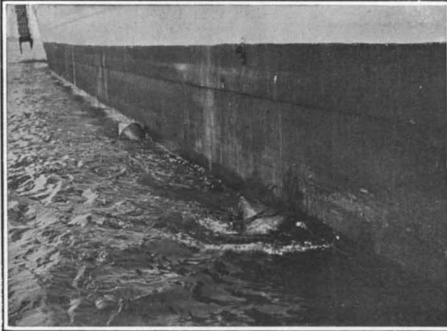
Floating the scrubber fore and aft. Ten tons of shell and weed were removed from one side alone of this steamer.
