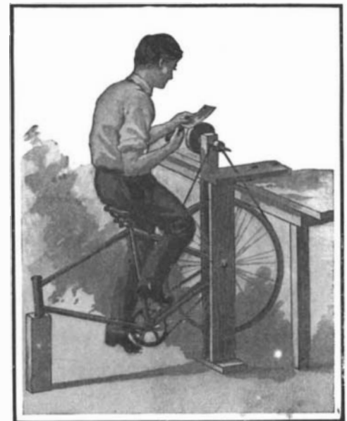
A SIMPLE FOOT-POWER GRINDER.
