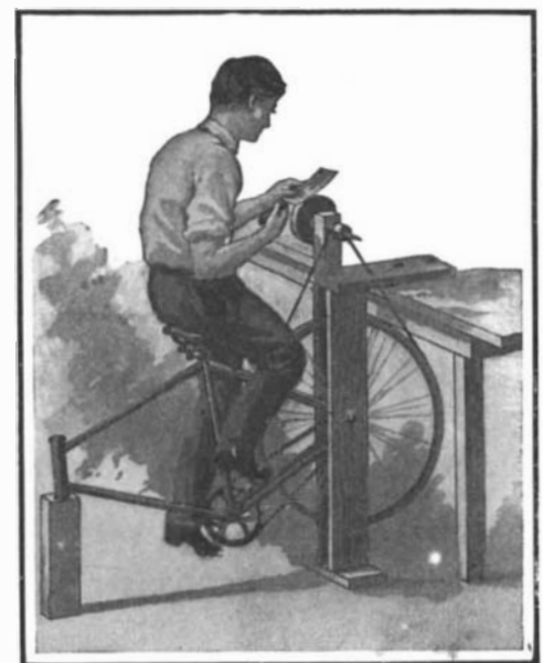
A SIMPLE FOOT-POWER GRINDER.
