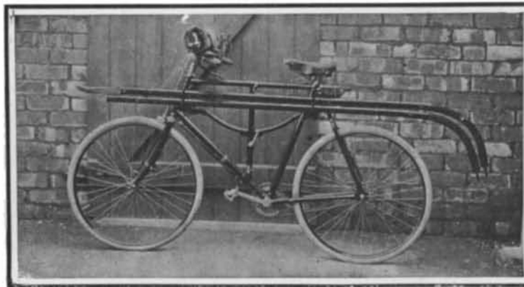
Simonis ambulance bicycle, which can be converted into an ambulance in three minutes.
