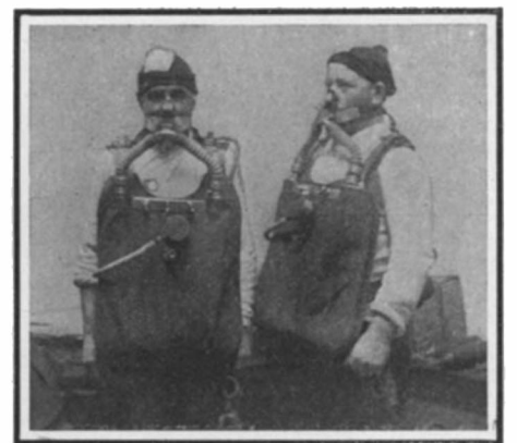
Two miners equipped with the Fleuss apparatus.
