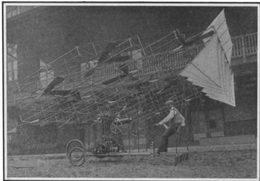
The machine is carried on bicycle wheels at its forward end and on skids at the rear end. On a control board in front of the aviator are a number of levers by means of which he can cut out any or all cylinders.
