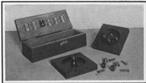
The Thermo-Electric Detector Taken Apart.
