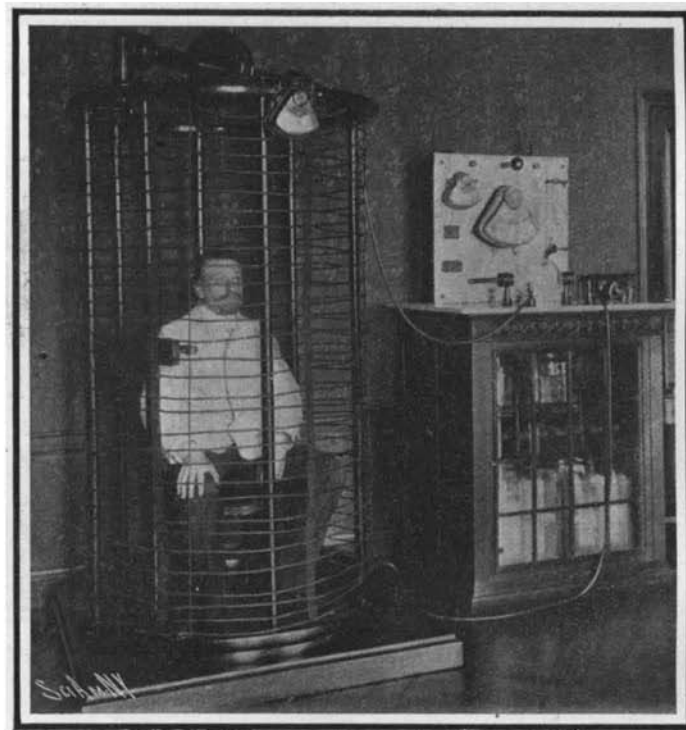
Fig. 1.—DR. MOUTIER'S APPARATUS FOR THE REDUCTION OF TERIAL PRESSURE BY MEANS OF HIGH-FREQUENCY CURRENTS.
