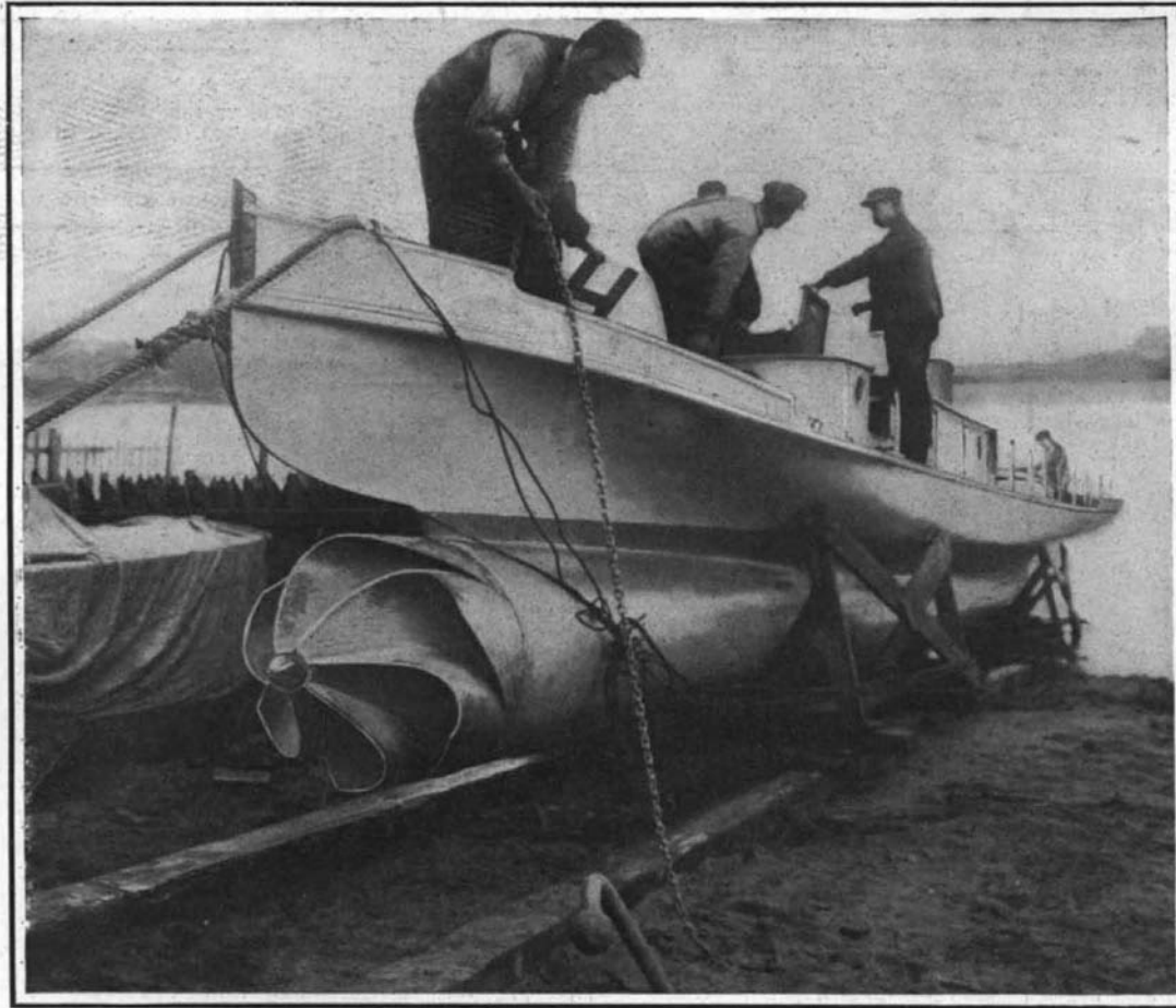
NOVEL MOTOR BOAT FITTED WITH A NEW FORM OF PROPELLER KNOWN AS A "TYPHONOID."
