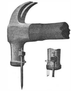
NAIL-HOLDING DEVICE FOR HAMMERS.
