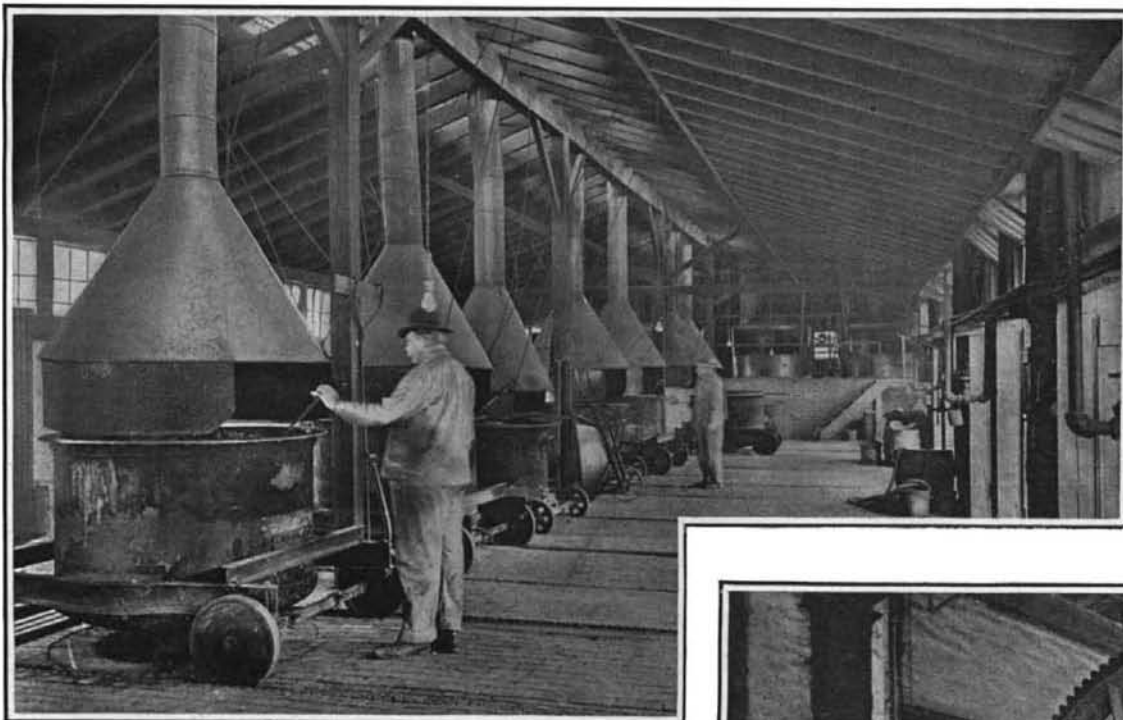
Section of Oil-Boiling Department. The Linseed Oil is Boiled to a Gelatin-like Consistency.
