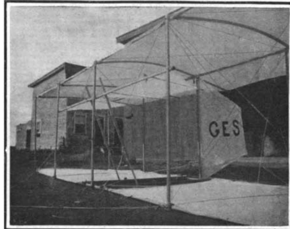
The Second Machine Equipped with the Final System Rudders. This System is to be Used on a Motor-Driven Flyer.
