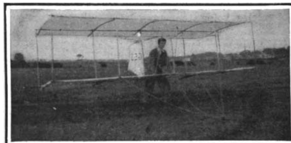
Starting a Flight of the Second Machine, Equipped With Final Arrangement of Rudders.
