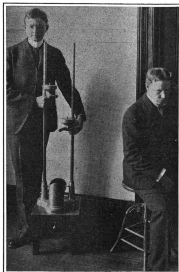
A Sonometer to Detect the Least Perceptible Difference in the Intensity of Sound.
