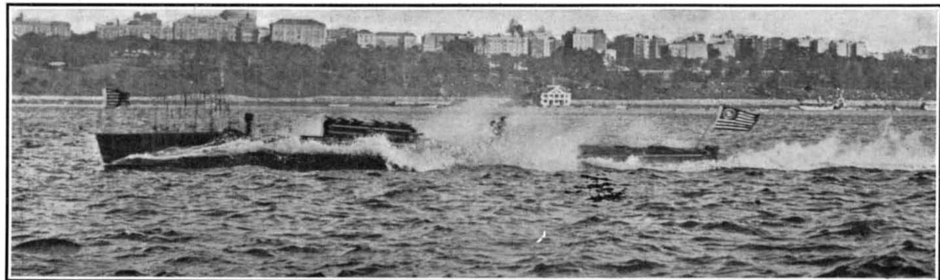
The 60-Foot Racer "Standard," Fitted With a 300 H. P. Double-Acting Standard Gasoline Motor. Average Speed in Mile Trials, 29.39 Miles per Hour.
