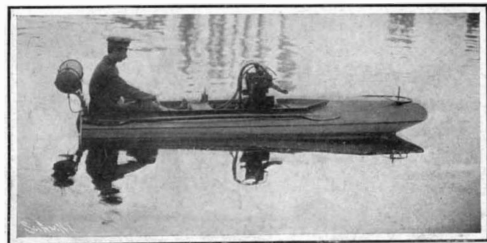
The "Ricochet-Nautilus," Which Has Attained a Speed of About 30 Miles an Hour With a 10-Horse-Power Motor. This Boat is About 11 Feet Long.
