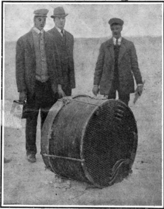
The Boiler of the Racer After the Accident.
