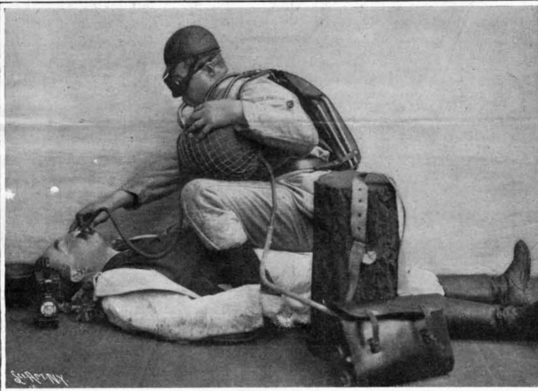
Reviving a Victim Overcome by Poisonous Gas by Means of Supplementary Oxygen Supply.
