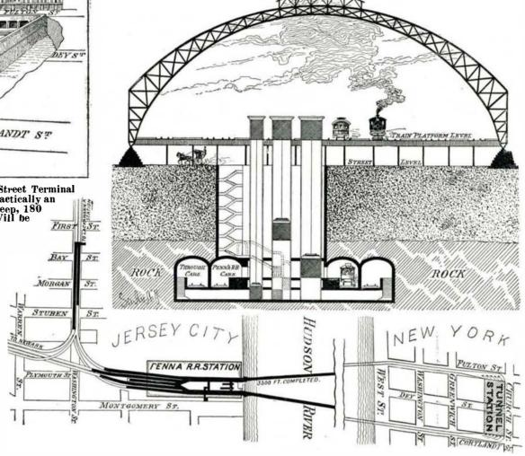
Plan and Section, Showing the Large Tunnel Station, 85 Feet Below the Pennsylvania Station, Jersey City, and Its Connection, by Tunnels Below the Hudson, with the Cortlandt Street Terminal, New York. The Heavy Black Lines Show, in the Plan, the Extent of the Completed Work.
