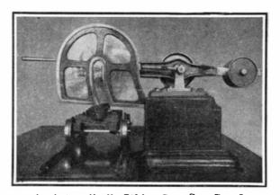
An Automatically Lifting Buzz-Saw Guard.
