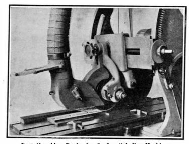
Dust-Absorbing Device for Surface-Grinding Machines.
