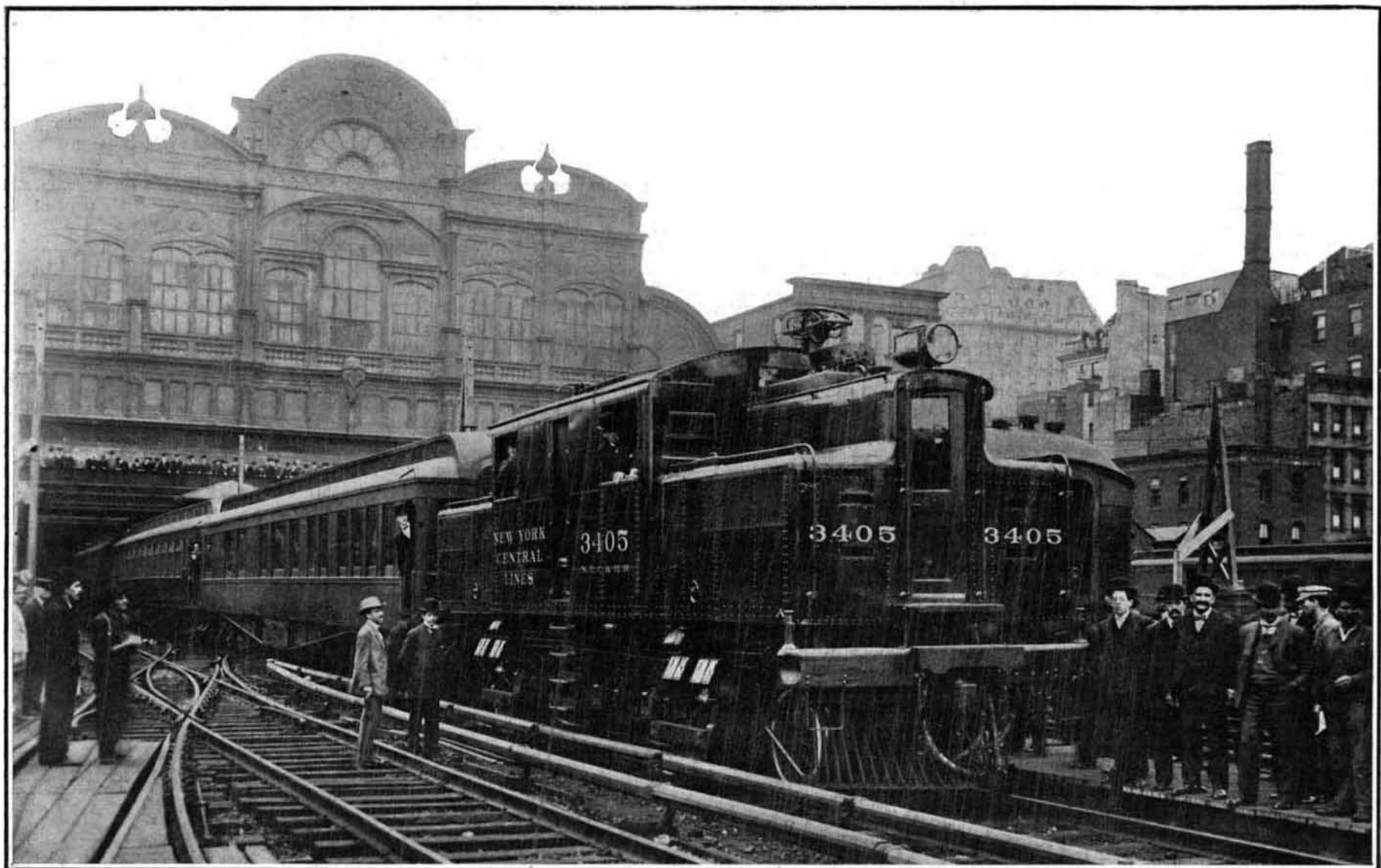
The locomotive, of 3,200 maximum horse-power, weighs 95 tons and can exert twice the horse-power of the express steam locomotives of the road.
