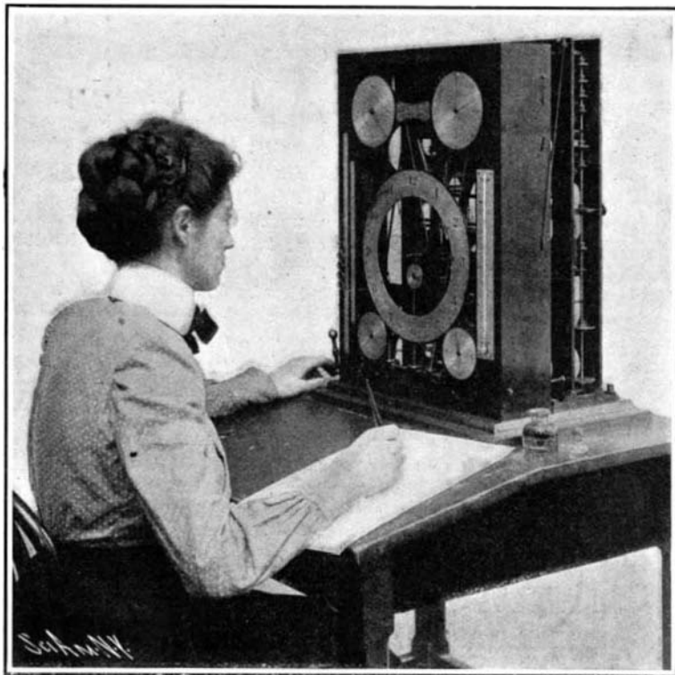
Operator Turning Indices to Determine the Height and Time of the Tide at a Future Date.
