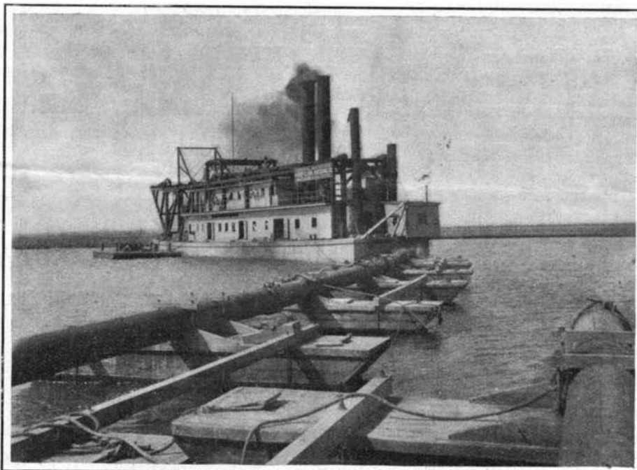
Stern View of the "Mackenzie," Showing Discharge Pipe.
