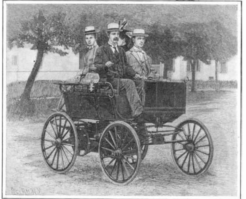
Mr. R. E. Olds' First Gasoline Machine, Built in 1896. The 5-horse-power motor and 3-speed transmission were arranged on the running gear.
