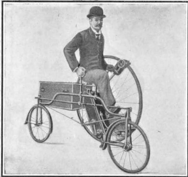
A. L. Riker's Electric Tricycle, Built Twenty Years Ago. A small battery motor drove the large wheel by friction.
