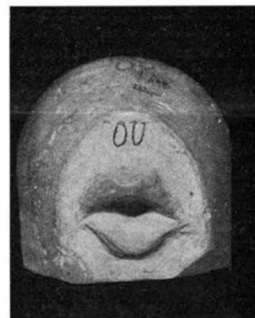
Fig. 4.—Artificial Mouth for Producing the Sound French "ou," (English "oo," as in "Moon.")
