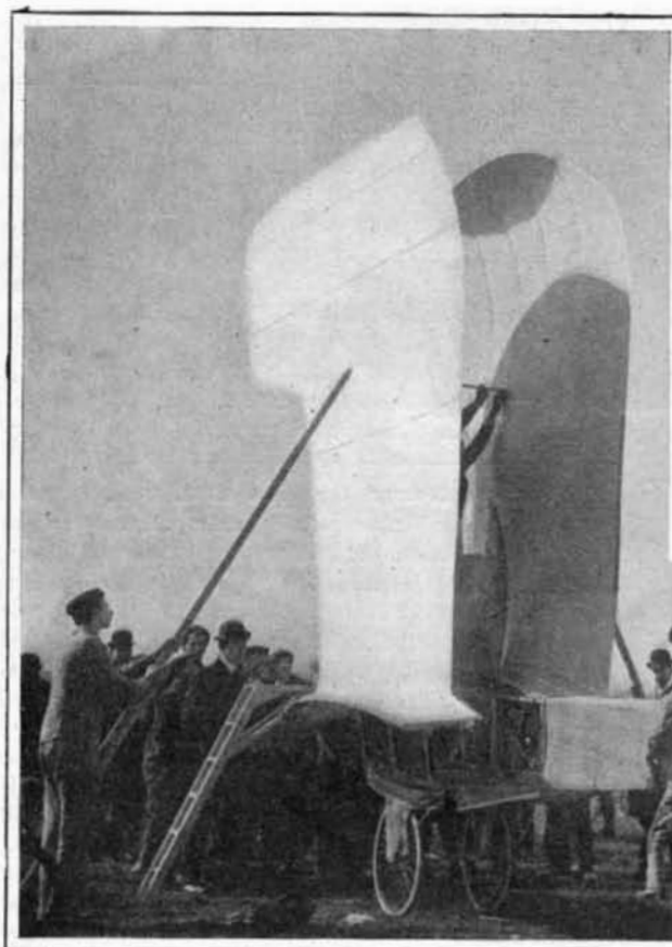
Attaching the Wings to the Aeroplane Upon Its Arrival at the Testing Place.
