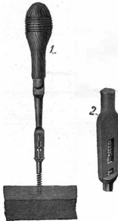
SCREW DRIVER WITH A CENTERING DEVICE.
