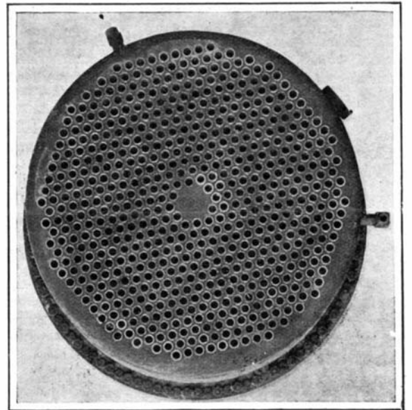
These Tubes Were Welded in Place by Means of the Oxy-Acetylene Blowpipe, With Which a Flame Having a Temperature of 7,000 Deg. F. Was Obtained.
