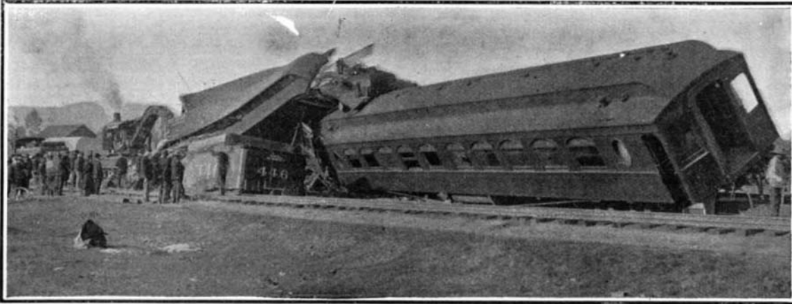
The Massive Vestibule Day Coach Crushed the Baggage and Smoking Cars into Fragments, but Itself Remained Practically Intact.
