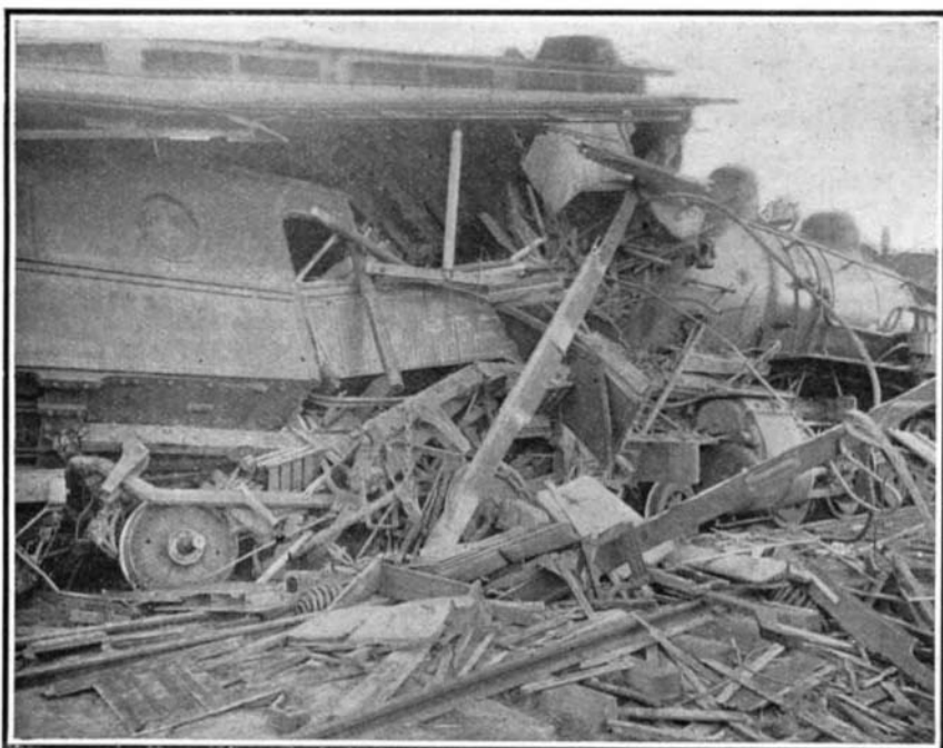
Wreckage of Baggage and Smoker After They Were Crumpled into Fragments Between Vestibule Coach and Freight Engine.
