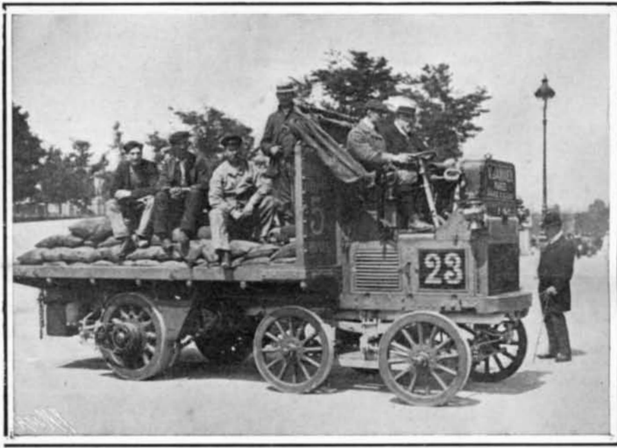
The 3-Cylinder, 24-Horse-Power Janvier Truck, Fitted with Novel Steering Bogie.
