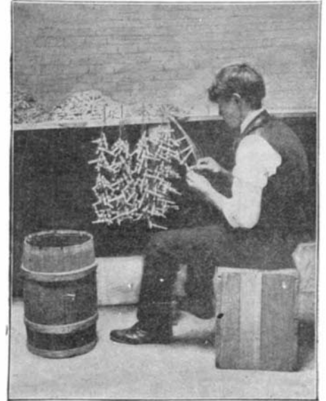
Old Method of Stringing Small Objects for the Plating Bath.
