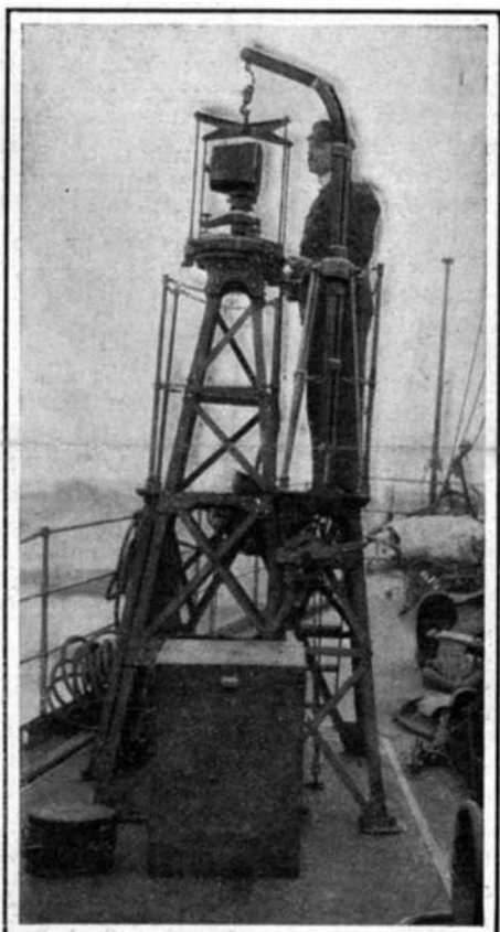
A Phototheodolite for Measuring Wave Lengths and the Coast Line.
