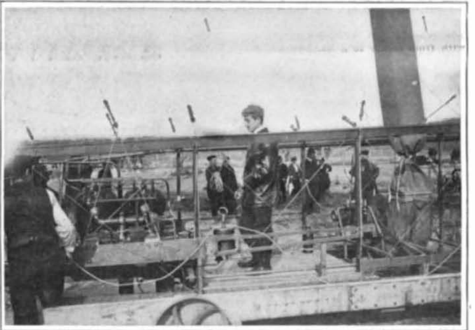
The Power Plant, a 70-Horse-power, 4-Cylinder, Water-Cooled Argus Motor.
