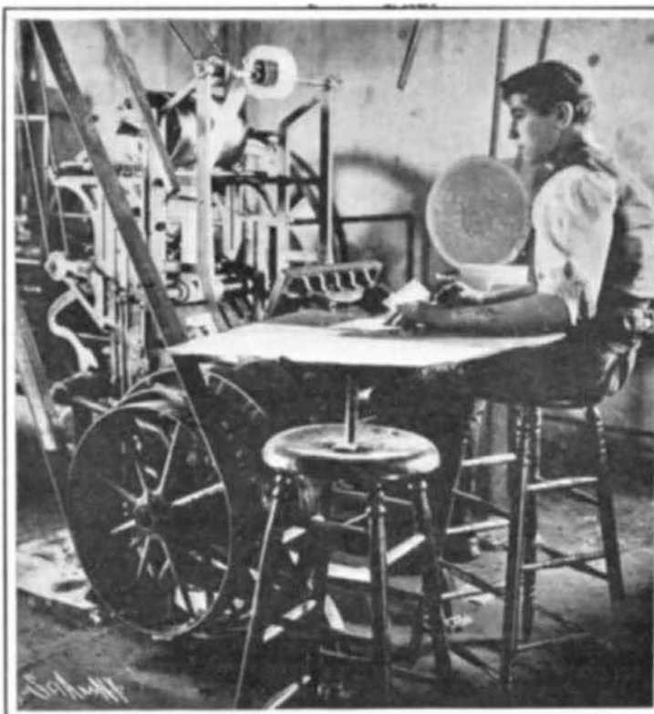
THE NEW PRESS FOR PRINTING AND EMBOSSEING STATIONERY FROM STEEL DIES. REAR VIEW OF THE MACHINE.
