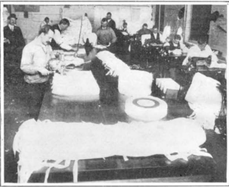
Making the Powder Bags in the Brooklyn Navy Yard. In the Foreground Are 6-Inch Bags for 6-Inch Shells.
