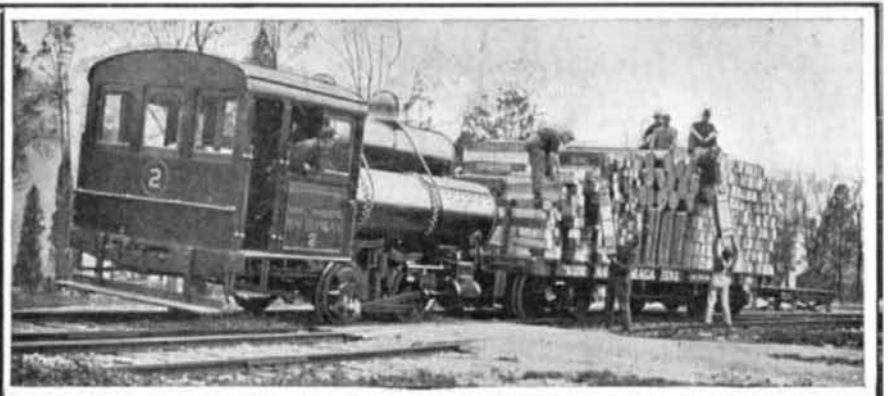
The Compressed-Air Engine for Handling Cars Loaded with Ammunition.
