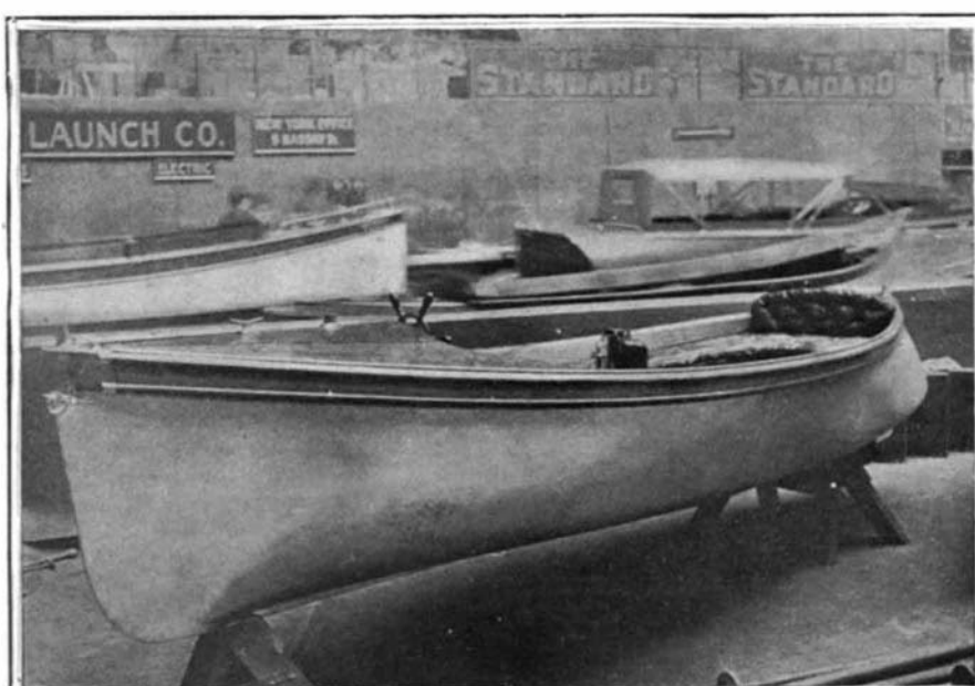
LIGHT, CHEAP, AND SERVICEABLE STEEL LAUNCHES FITTED WITH AIR TANKS WHICH MAKE THEM UNSINKABLE.
