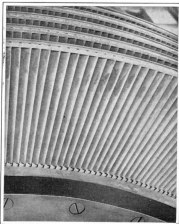
A Portion of the Spindle, Showing the Blading.
