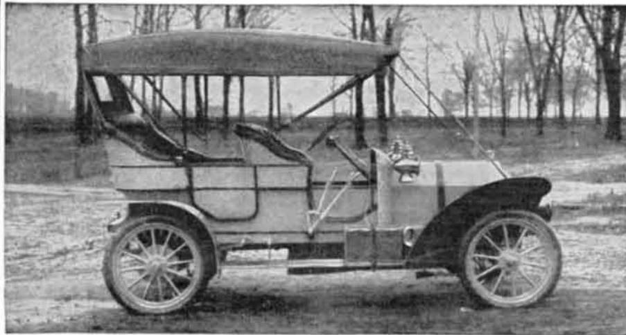
MODEL S, 4-Cylinder, 26-28 h. p. Price $2250 (with complete lamp and horn equipment.)
