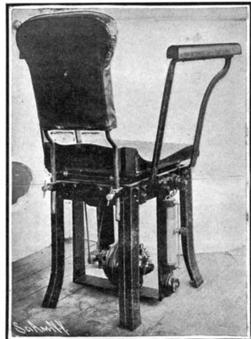
A Chair Designed to Prevent Seasickness. The Seat is Movably Arranged and is Reciprocated Rhythmically by Means of an Electric Motor Connected by Means of a Belt with an Eccentric Actuating the Seat.
