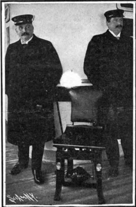
A Chair Designed to Prevent Seasickness. The Seat is Movably Arranged and is Reciprocated Rhythmically by Means of an Electric Motor Connected by Means of a Belt with an Eccentric Actuating the Seat.
