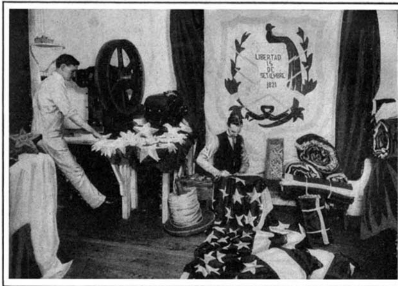
The Star Cutting Machine; Sewing On a Halyard Bend.
