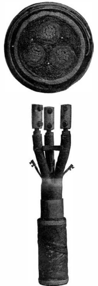
Sections of High-Tension Cable.
