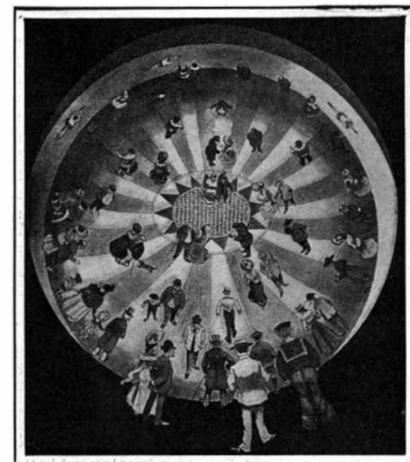
Fig. 5.—This picture shows how the rotating parabolic floor will appear to an observer standing on its outer edge. The cyclists are apparently riding on a vertical surface.
