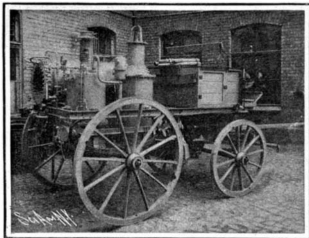
Fig. 1.—Portable Military Sterilizer. Capacity, 500 Liters per Hour.
